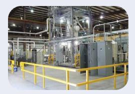
The instrumentation and automation equipment are from the same manufacturers and the same models as those commonly found throughout the refining and chemical process industry. Control valve stations, pump configurations, piping and structure are all built to industrial standards. Each unit is provided with a curriculum of over 100 specific real world procedures and exercises.
